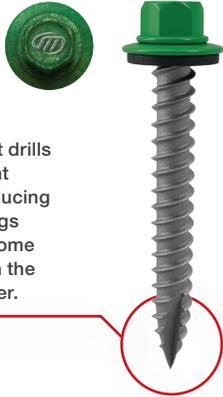
Type 17 point drills with no “point walking,” reducing metal shavings that can become embedded in the rubber washer.
