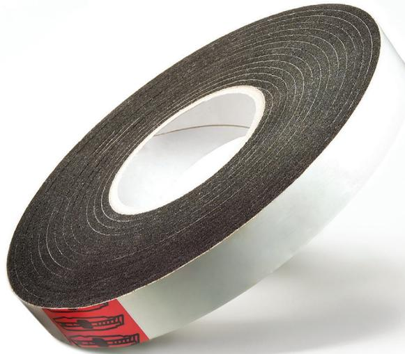
**Automatically expands to fill any-shaped gap in the construction of metal buildings, doors and windows, concrete, wood and more.** X-Seal™ comes compressed at just one-quarter inch, on an easy-to handle roll. Cut the desired length of X-Seal, place X-Seal into the gap opening—even one with irregular hips and valleys—and remove the protective release paper. Now watch X-Seal slowly expand to completely fill and seal the gap.
