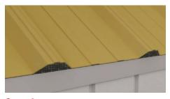
Step 3: Place the roof panel over pre-cut closure configuration for a snug fit. Attach panel over closure with Marco QuikGrip<sup>™</sup> or QuikDrill<sup>™</sup> fasteners.
