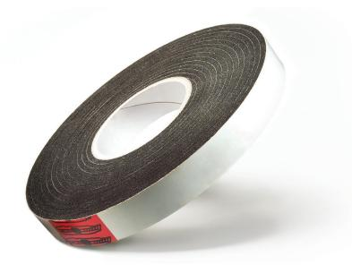
Automatically expands to fill any-shaped gap in the construction of metal buildings, doors and windows, concrete, wood and more. X-Seal™ comes compressed at just one-quarter inch, on an easy-to handle roll. Cut the desired length of X-Seal, place X-Seal into the gap opening—even one with irregular hips and valleys—and remove the protective release paper. Now watch X-Seal slowly expand to completely fill and seal the gap.
